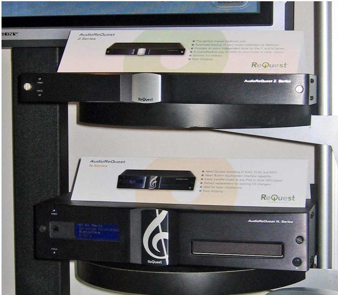
Figure 23 - ReQuest audio distribution via Ethernet
